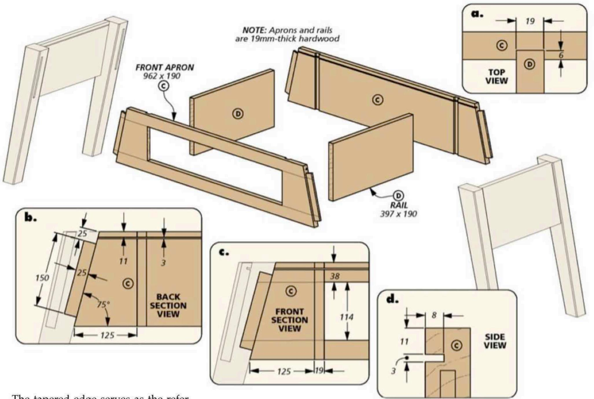
The tapered edge serves as the reference surface for mortises with a consistent depth.
