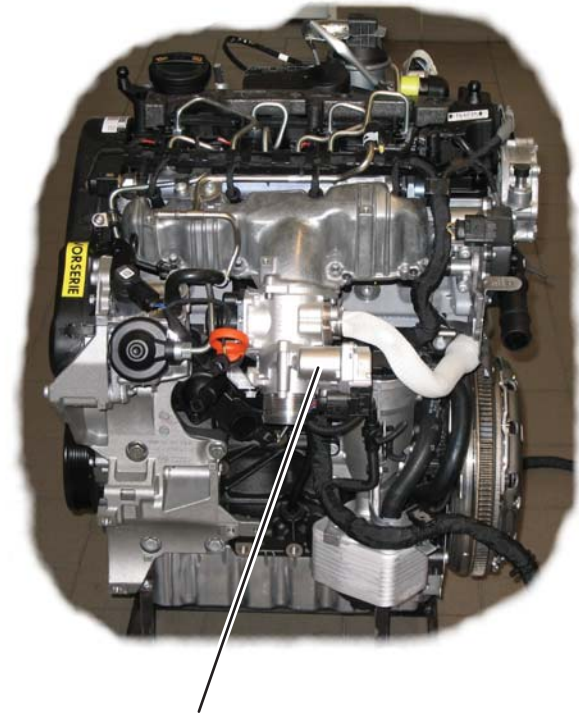
Throttle Valve Control Module J338 with Throttle Position (TP) Sensor G69
