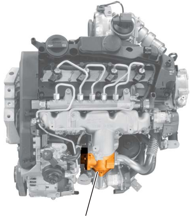
Exhaust Gas Return Valve with EGR Potentiometer G212 and EGR Vacuum Regulator Solenoid Valve N18
