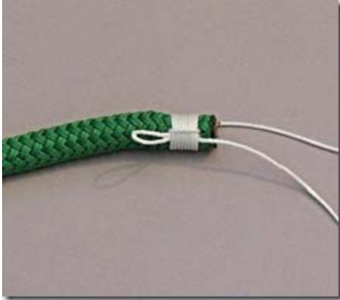
Whipping the end of a double braid line – Step 7
