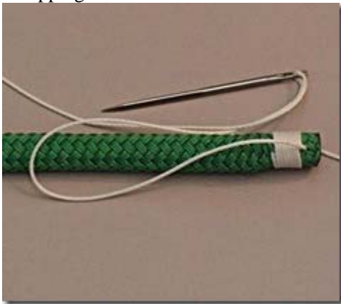
Whipping the end of a double braid line – Step 7
