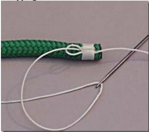
Whipping the end of a double braid line – Step 8
