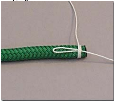
Whipping the end of a double braid line – Step 2
