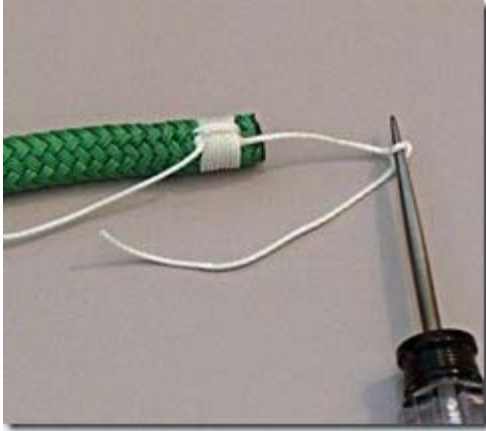
Whipping the end of a double braid line – Step 10
