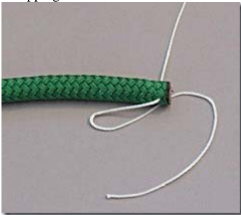
Whipping the end of a double braid line – Start
