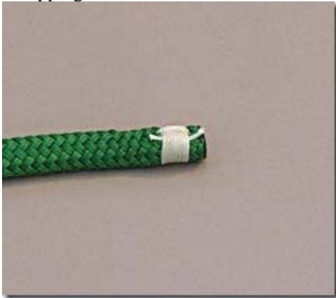
Whipping the end of a double braid line – Step 11
